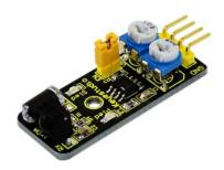
Infrared obstacle avoidance sensor is equipped with a pair of infrared transmitting and receiving tube. When infrared ray launched by the transmitting tube encounters an obstacle (its reflector), the infrared ray is reflected to the receiving tube. The reflecting light strength is then converted into current signal. When it detects an obstacle, it outputs low level signal 0; when no obstacle is detected, it outputs high level signal 1.
