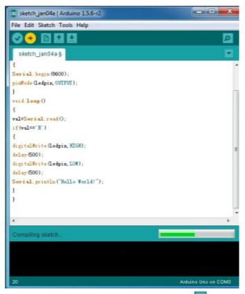
After uploading is done, open "serial monitor ", enter "R"; click "Send", the serial monitor will display "Hello World!" and the D13 LED will blink once.
